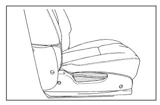
3. Lift the recliner lever, located on the outboard side of the seat, up fully and fold the seatback forward until it disengages.
